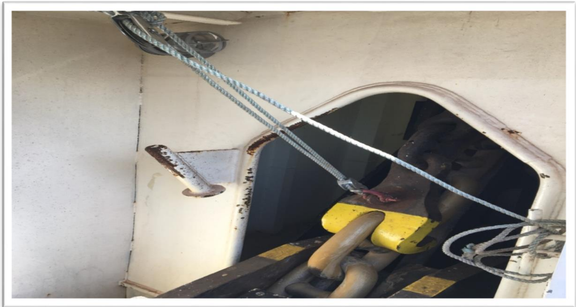
Figure 4-5 In this image the starboard claw is engaged on the anchor chain. When the not engaged, it is lifted up by pulley and tied to a cleat on the bulkhead.
