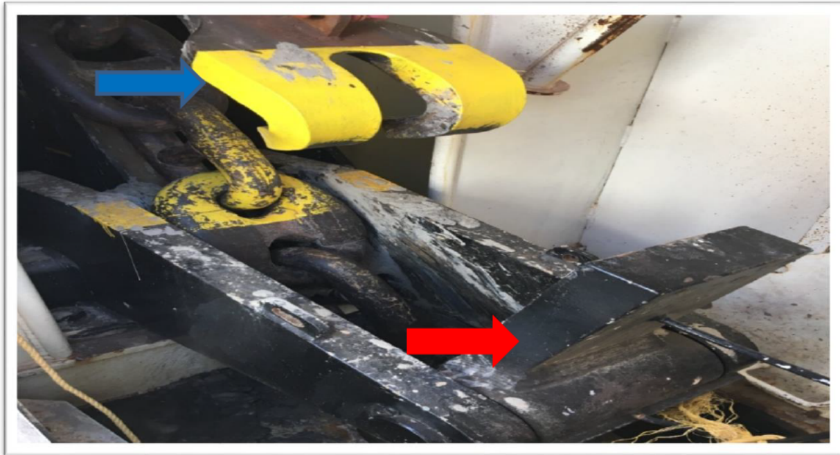
Figure 4-4 The starboard claw and paw on the ERIE TRADER. In this image both devices are un-engaged. The claw (indicated by blue arrow) is tied off to the cleat on the bulkhead. The paw (indicated by red arrow) is pulled back and into an upright position.
