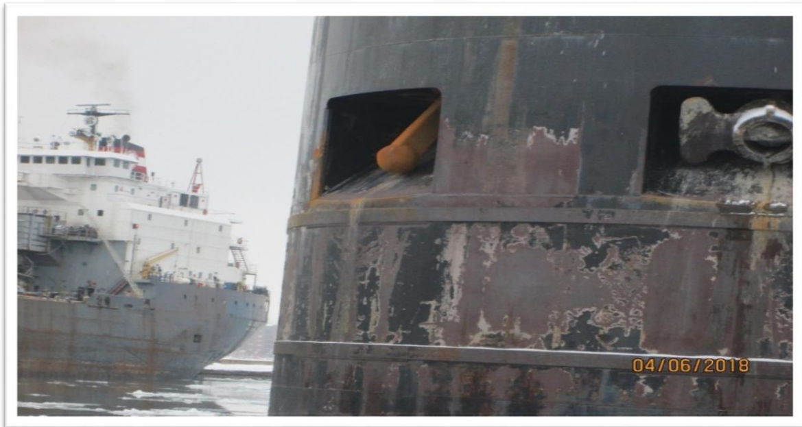
Figure 4-11 ERIE TRADER missing flukes on starboard anchor 6 April 2018 at South East Pier St. Marys River
