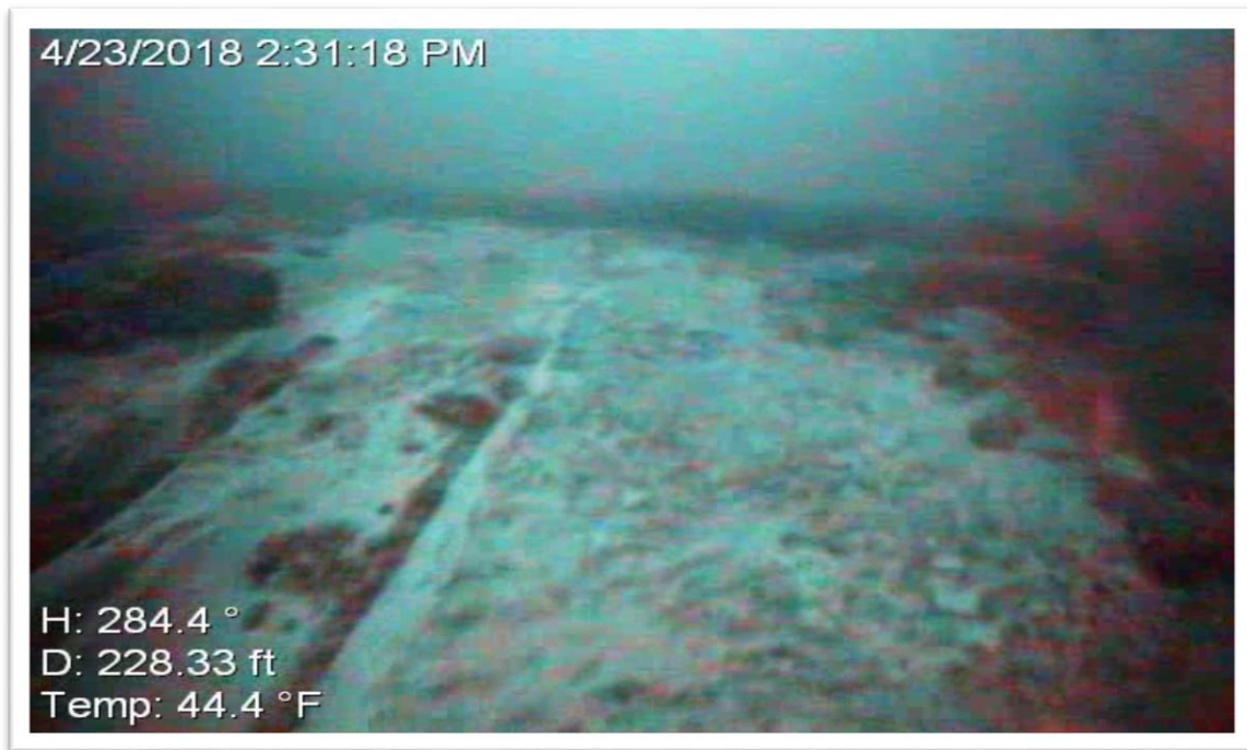
Figure 4-13 Drag marks in the seabed just before the Line 5 Pipeline. The marks depicted were not measured. ROV Image provided by Enbridge Inc.
