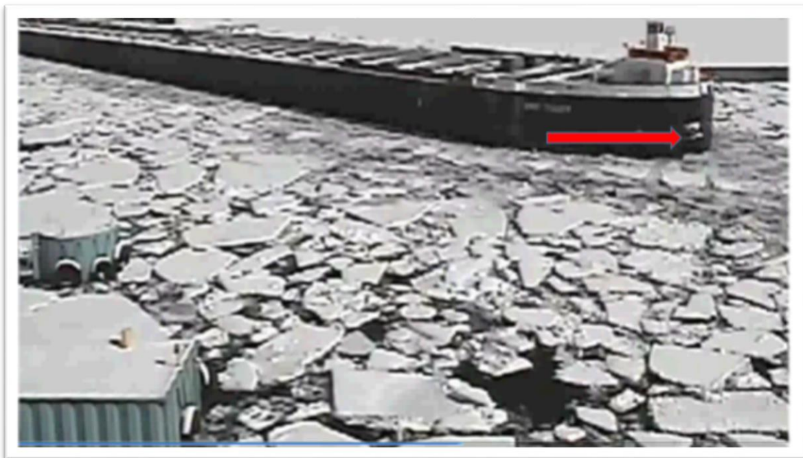
Figure 4-7 The ERIE TRADER in the St Marys River at Rock Cut west of Neebish Island on 1 April 2018. Image captured by Coast Guard VTS cameras depicts significant ice conditions. Red Arrow points to ice on the starboard anchor hanging below the anchor pocket.
