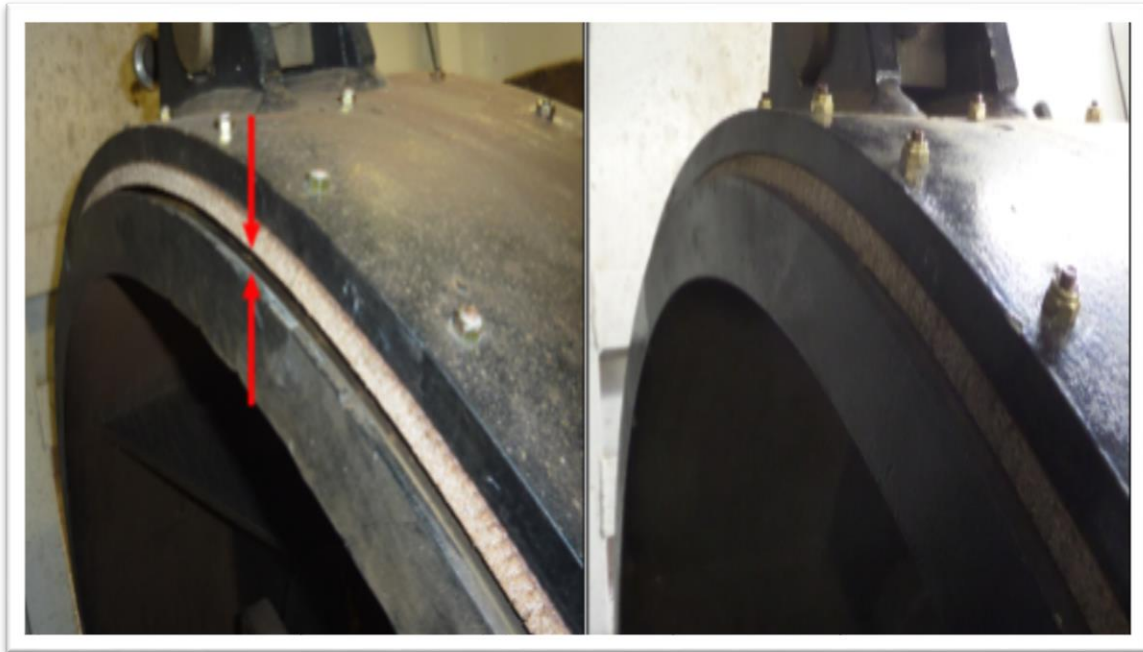
Figure 5-1 Left: Post accident photo of the upper brake band liner for the starboard anchor with the brake engaged. The red arrows highlight the noticeable gap at the top between the drum and liner.
